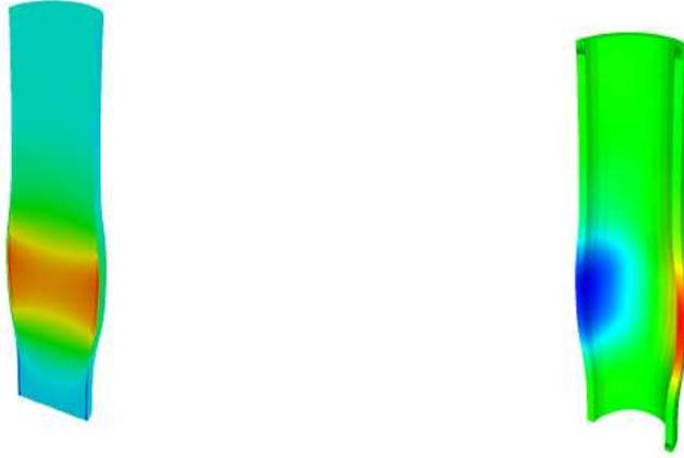
FIG. 7 – Solution of the 3D model at  $t = 50.10^{-4}$  (left : fluid velocity, right : wall displacement)
